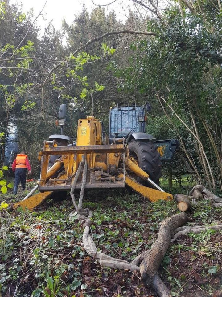
Ropes and cables are attached so that Neil Gosling controlling the telehandler can slowly lift and pull each part of the trunk back to the river bank.
